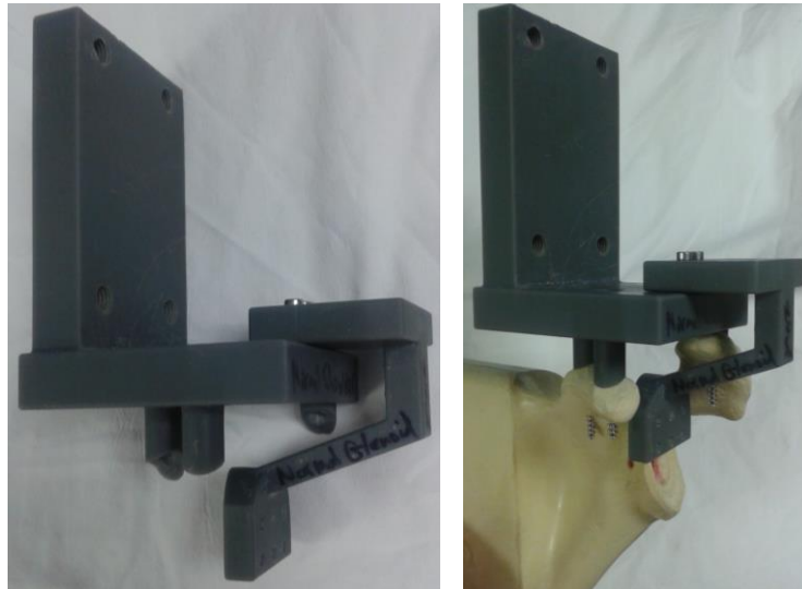
Figure 3-4: Patient specific mount assembly and attached to the sawbone model
