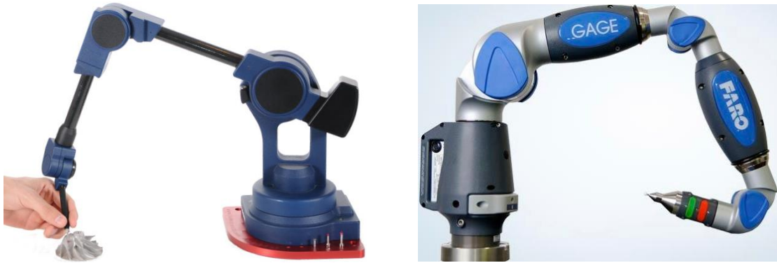
Figure 1-6: Serial linkage arms: Microscribe (left) 4 , FARO GAGE arm (right) 5
